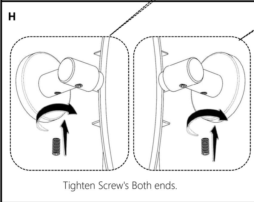
Tighten Screw's Both ends.
