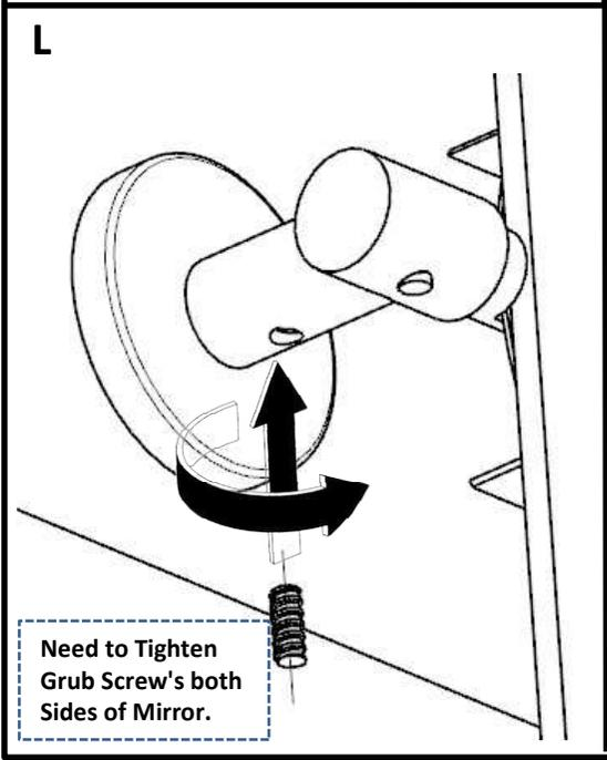
Need to Tighten Grub Screw's both Sides of Mirror.
