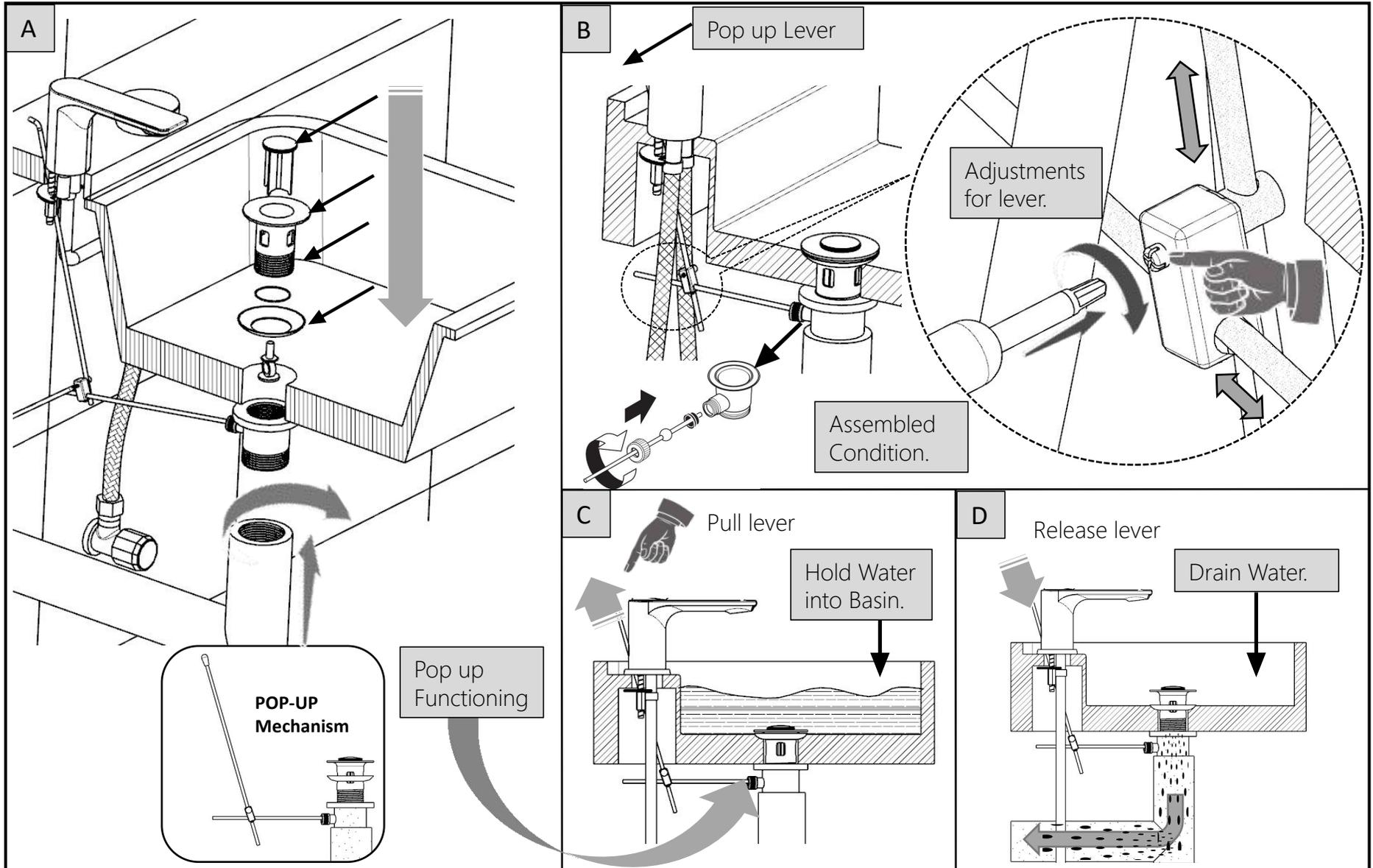
Note: This Installation Method is applicable for Single Lever Basin Mixer with Pop-up Waste System.
