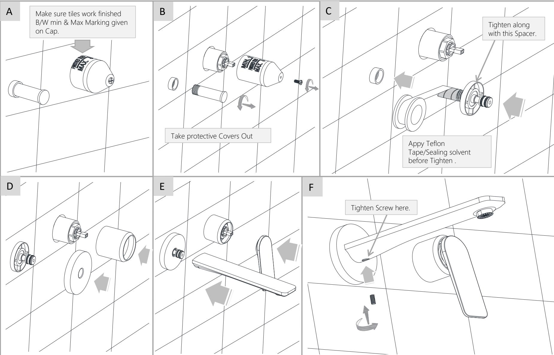
**Note:** THIS INSTALLATION MANUAL CAN BE REFERRED FOR ALL EXPOSED PART KIT OF SINGLE LEVER BASIN MIXER WALL MOUNTED WITHOUT WALL FLANGE.
